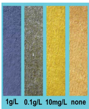
Fig. 5 The color changes of the test papers for detecting fluoride ion in neutral aqueous solution with different F^- concentrations.
